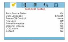
**Auto Source Detect :** The monitor will auto detect the video source when power ON.
